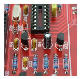
After all the welding jobs have been done, please connect the electric power instead of connecting Atmega328 and LCD(9V battery or external 5.5-12V DC power, outside -, inside +), and measuring the voltage of the pin7 and pin22 on the IC plug by using the multi-meter, and the voltage should be +5V(the button should be pushed when measuring), which means the circuit and power are working in normal condition.
