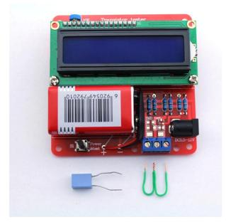
The test 4 will finish only automatically if you separate the test ports (release connection). You should not touch to any of the test ports or connected cables when calibration is done. But the equipment should be the same, which is used for further measurements. Otherwise the zero offset for capacity measurement is not detected correctly. The resistance values of port outputs are determined at the beginning of every measurement with this option.
