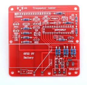
Next, weld the other electrical components based on , and please be aware of the type and direction of the transistor, and the blue wiring terminal is optional:
