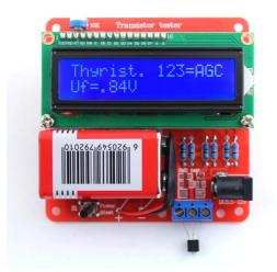
Thyristors and Triacs can only be detected, if the test current is above the holding current. Some Thyristors and Triacs need as higher gate trigger current, than this Tester can deliver. The available testing current is only about 6mA! J-FET measurement(2SK30A):
