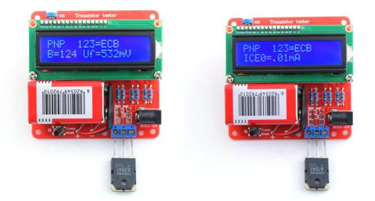
Display the Collector cutoff current Iceo with currentless base (10uA units) and Collector residual current Ices with base hold to emitter level . This values are only shown, if they are not zero (especially for Germanium transistors).
